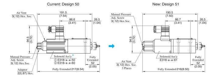
★ The solenoid assembly current design comes in two types: ① E318-50 design and ② 60 design. See the figure on the left for an external view of type ① . See the figure on the right for type ② .
