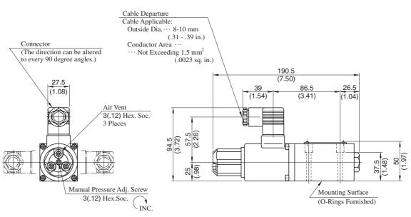
Note: For valve mounting surface dimensions, see the dimensional drawings of sub-plates (P.356) in common use.
